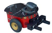
Fig. 5: A typical prototype of Pioneer 2-DX robot with gripper.
