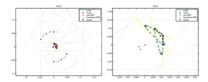
Fig. 2. Footprints with center of mass trajectory, theoretical and real zero moment points in rotation motion of 60[deg] about the middle of ankle joint centers. Model of linear inverted pendulum. The right view is a zoom of the COM trajectory from left view.
